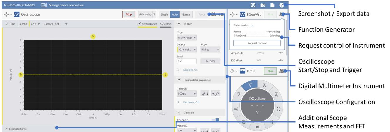
Figure 6. NI ELVIS III Oscilloscope Soft Front Panel
